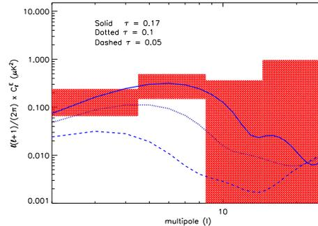
Figure 1: Errors (68% C.L.) on the power spectrum  $C_l^E$  achievable by SPOrt in the case of  $\tau = 0.17$ .
