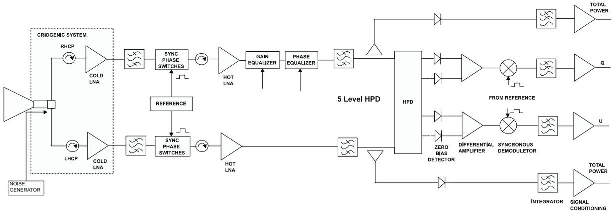
**FIGURE 3.** Block diagram of the BaR-SPOrt radiometers.
