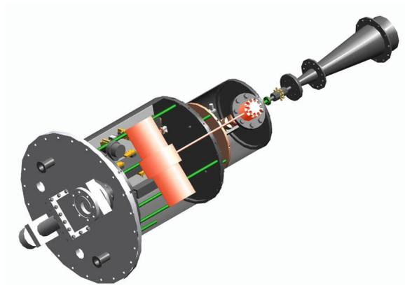
**FIGURE 6.** The radiometer inside the cryostat.
