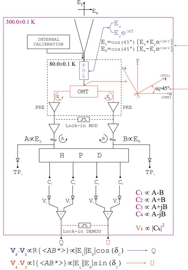
**FIGURE 4.** Scheme of the radiometers with the propagation of the fields collected by the feed horn.
