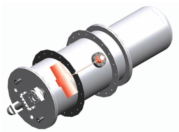
**FIGURE 5.** The cryostat housing the 32 GHz radiometer of BaR-Sport with the closed loop cryocooler visible in the foreground.
