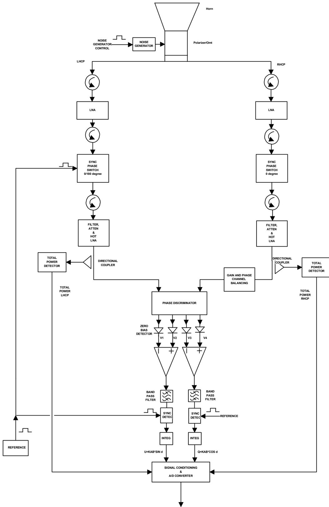
Figure 4. Block diagram of SPOrt correlation radio polarimeters.
