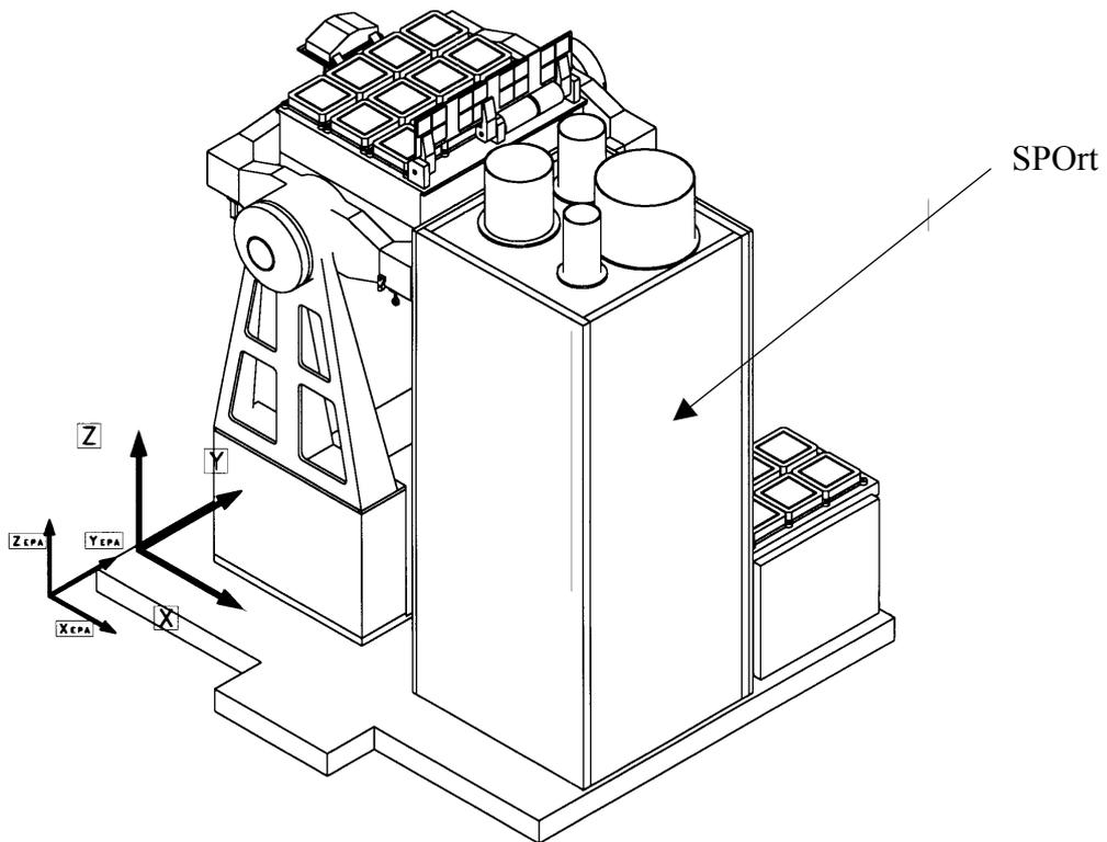
Figure 3. The SPOrt payload accomodation on the EXPA together with EXPOSE
