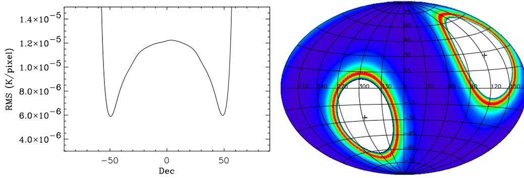
Figure 2. Expected sensitivity for 1.5 years SPOrt lifetime across the sky for the 90GHz channel (left panel) and the sky coverage in galactic coordinates (right panel). Colors refer to different integration time (from 30 to 120 Ksec).
