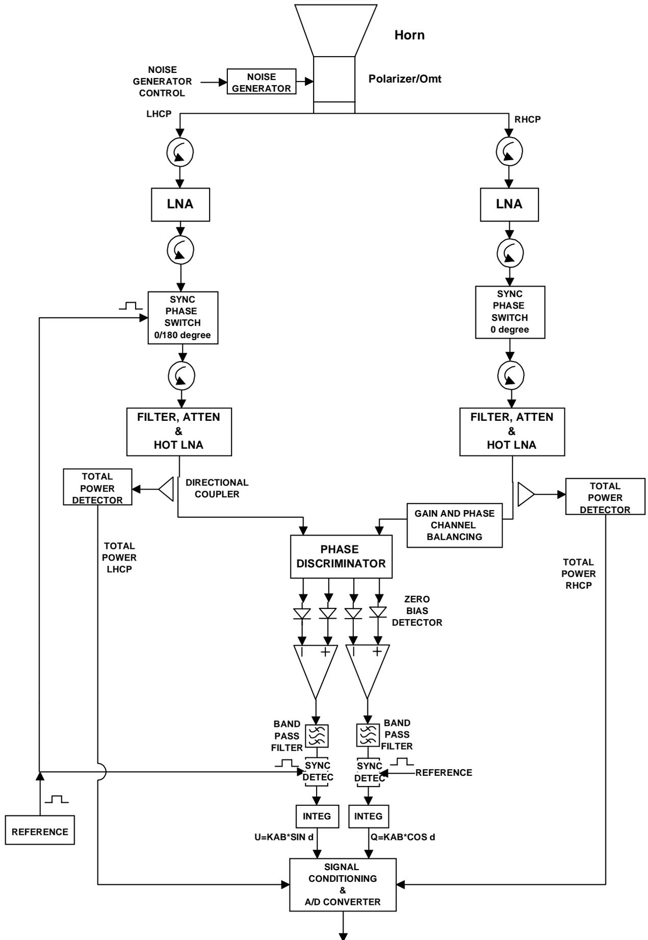
FIGURE 1. Schematic block diagram of the SPOrt radiometers.
