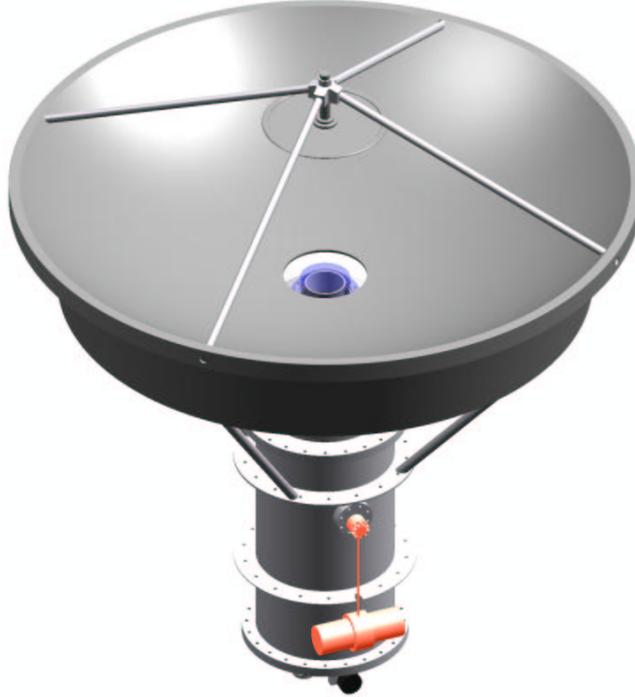
**Figure 2.** View of the 32 GHz receiver coupled to the 1.8 m Cassegrain optics. The dielectric window closing the vacuum chamber of the receiver is visible at the horn mouth.
